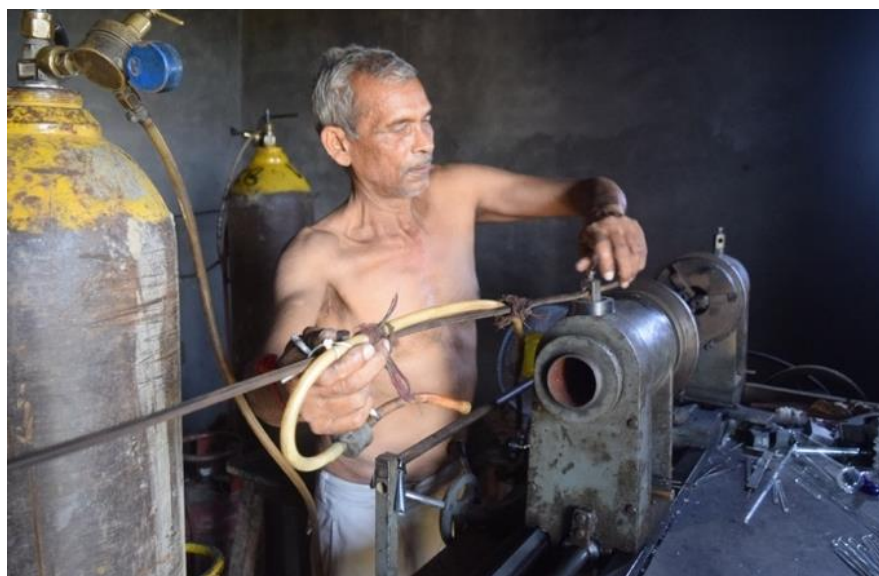
Figure 12: Artisan (Debendra Ji) demonstrating glass lathe machine in his studio.
